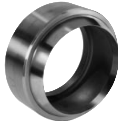
A helicopter swash plate bearing. The teflon liner in the I.D. of the outer race and the bore of the ball accommodates misalignment and linear motion.
